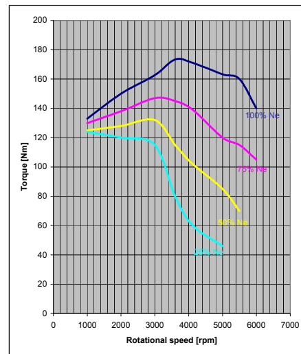
Fig. 3. Characteristics of torque for increasingly smaller partial powers respectively for full value, 3/4, 1/2 and 1/4 of rated power in function of rotational speed
